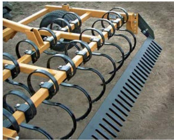
Two rows of heavy duty S-tine shanks.
