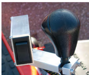
Rocker switch allows the operator to control grapple movement with the touch of a finger.
